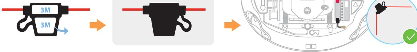
**Mount the Fuse Holder:** Remove the stickers from the fuse holder and stick them onto a dry, debris-free plastic surface. Apply some pressure to ensure it adheres firmly.
