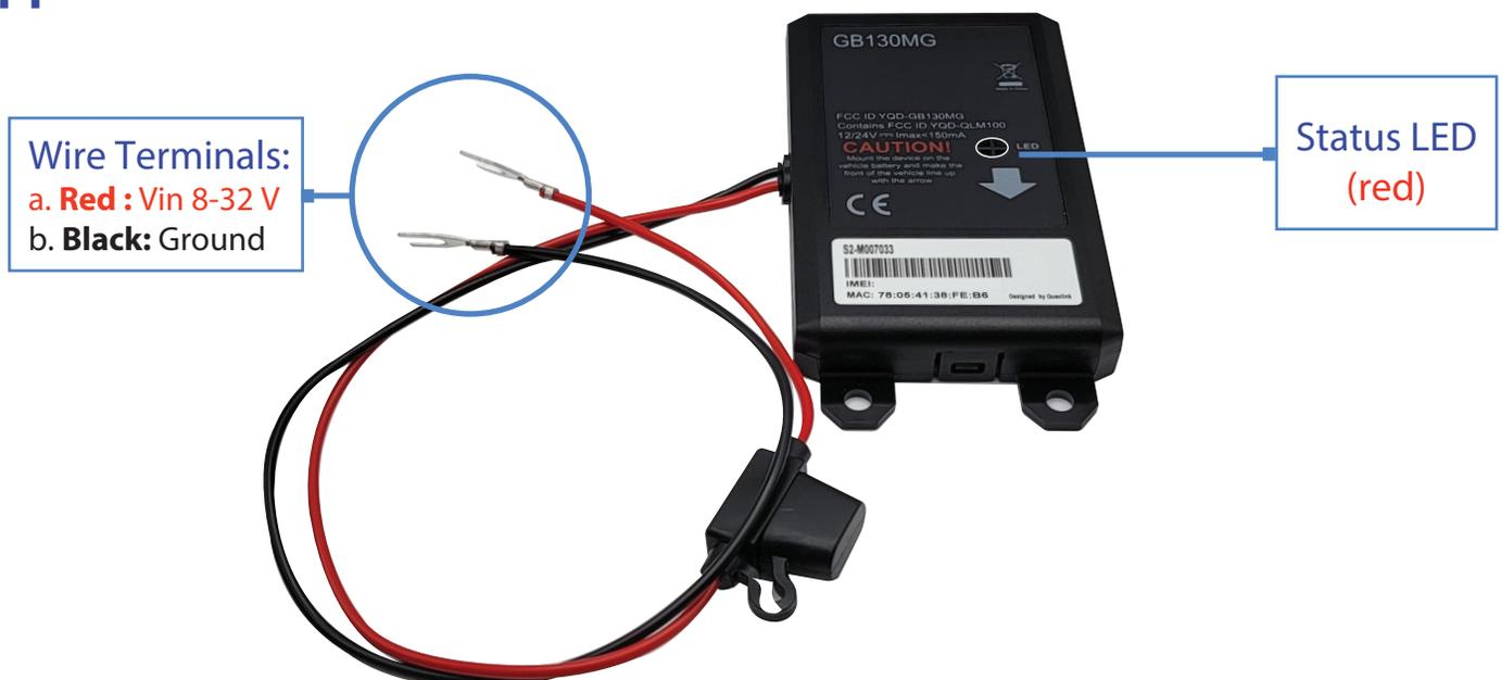
**Status LED (Red):** The following behavior is valid for the first 30 minutes following proper installation. After this period, the red LED will turn off.
